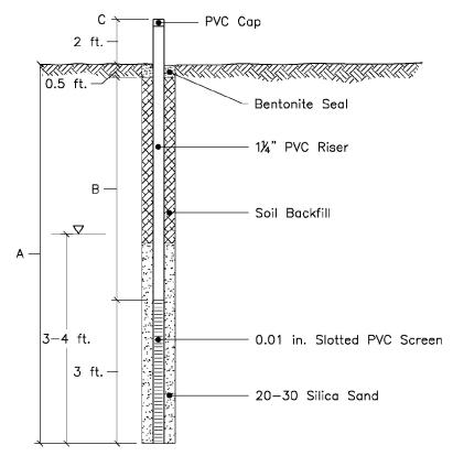
Figure 3-19. Construction Details for Groundwater Monitoring Wells.
