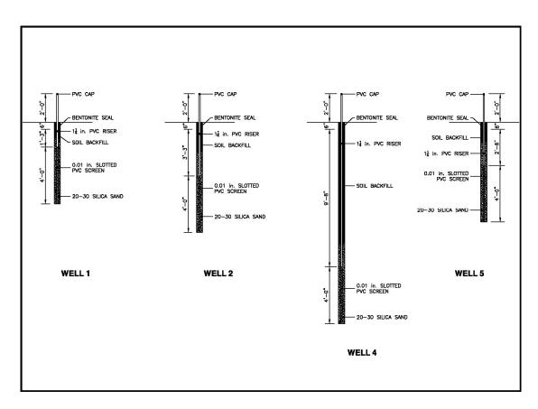
Figure 3-20. Construction Log for the Shallow Monitoring Wells.
