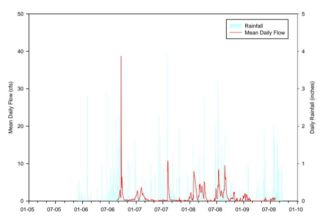
Figure 2-14. Historical Discharge Data for the Innisbrook Canal at Monitoring Site 02-09.
